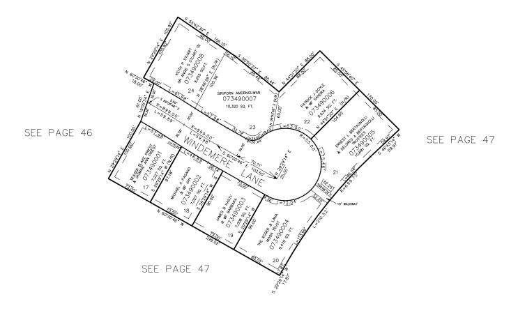
7' UTILITY AND DRAINAGE EASEMENT EACH SIDE OF PROPERTY LINE AS INDICATED BY DASHED LINES UNLESS OTHERWISE SHOWN.
